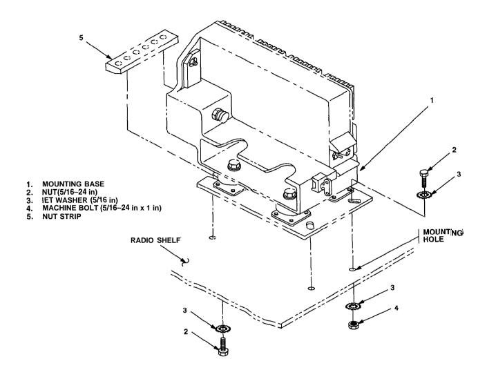
Figure 5-6. MT-6353/VRC Mounting Base Installation
