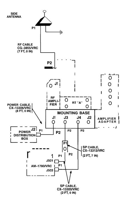
Figure 5-7. Cable Diagram: For AN/VRC-87/88/90 Series or AN/VRC-89/91/92 Series. Continuted
