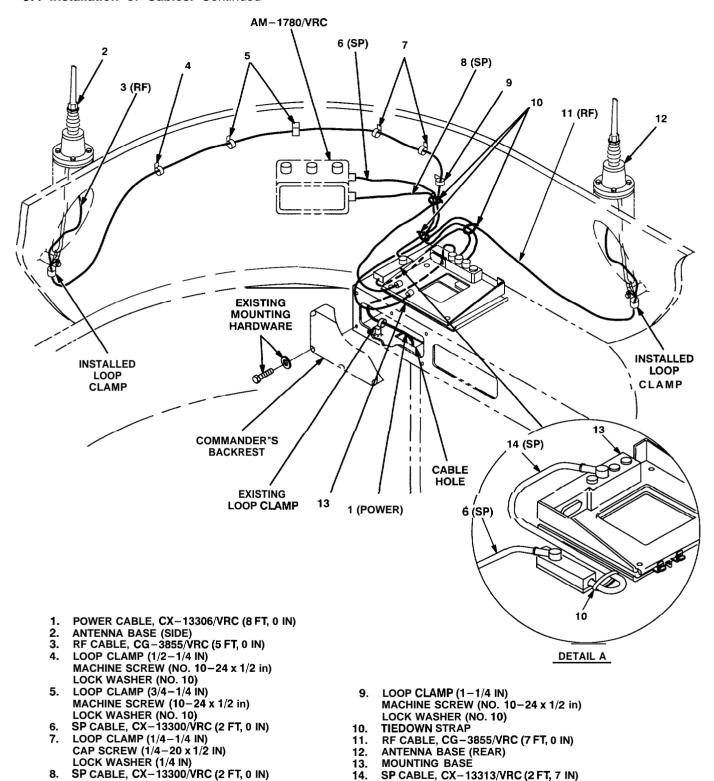
Figure 5-5 (2). Cable Installation: Turret Interior
