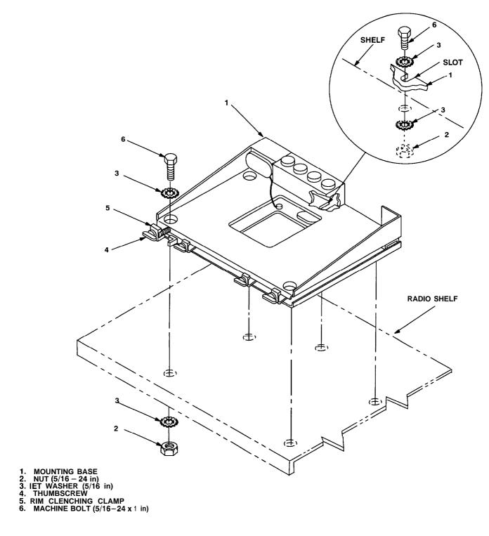
Figure 5-4. Mounting Base Installation
