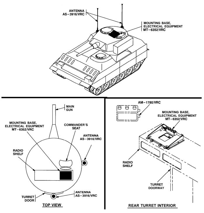
Figure 5-1(1). MK and Radio Installation: MK Equipment Locations
