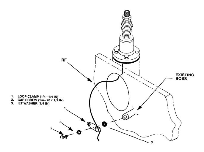
Figure 5-5 (3). Cable Installation: Loop Clamp Installation
