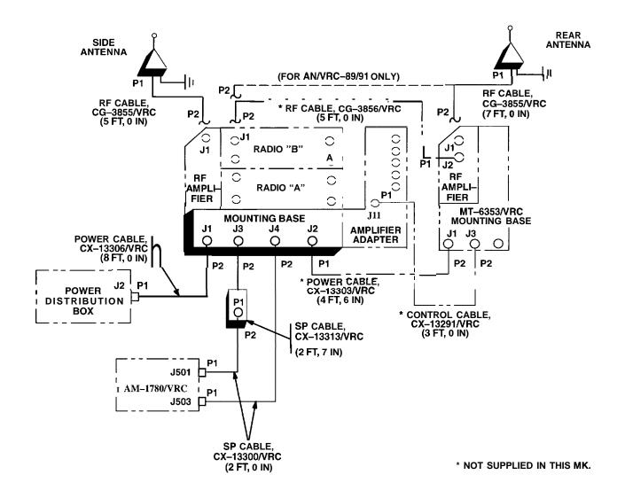
Figure 5-7. Cable Diagram: For AN/VRC-87/88/90 Series or AN/VRC-89/91/92 Series.
